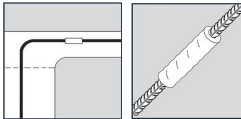
**Mechanical Connection and Anchorage of Reinforcing Steel Bar by means of Extruded Couplers
