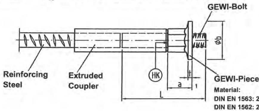
**At Tensile- and Compressive Load with Anchor Plate and Anchor Nut**
